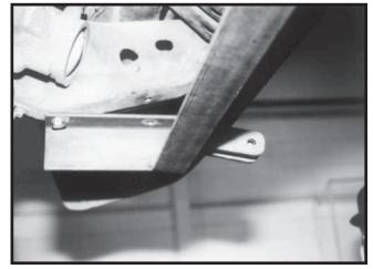
Install base plate with rear bolts snug so front ears touch Air dam/Valance. NOTE: Some bolts may need to be put back in so it is stable for marking and cutting of slots.
